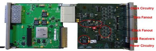
The CC system is responsible for the synchronisation of the detectors and the DAQ system to the general EuXFEL timing. The EuXFEL facility will generate coherent and intense X-ray flashes with a ~4.5 MHz bunch frequency. The Timing Receiver (TR) board housed in the same crate as the CC system delivers the bunch clock to the CC through the MTCA.4 backplane.
