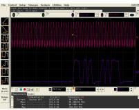
The tests were performed using Ethernet cables of lengths 10m, 15m, 20m, 30m and 50m. There were no errors observed during a period of more than 24 hours with the CAT6 SFTP cables up to 30m. If there is a need to support a 50m cable length MLVDS drivers are going to be tested for data and clock transmission.
