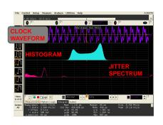
Further tests involved applying filtering on the 3.3 V rail to reduce the jitter readings. In order to do this, LTM4600EV was soldered on a small PCB and this PCB is attached to the CC RTM by cables so that it received the 12V RTM power from the DAMC2. The most promising jitter readings were obtained when a LC filter (1uH/1UF) is attached to the output of the DC/DC converter in addition to the required capacitors.
