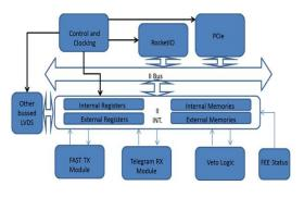
around a bus/register structure called the II Bus, whose registers are accessed through either the PCIe link to the crate processor or the blocks attached to the bus. The EuXFEL central software system controls the CC system through the PCIe link.
