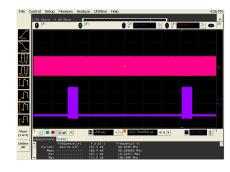
The receiving circuitry transfers the data to the FPGA on the receiver card and the data is compared to the data generated on the receiver card in tandem. In the receiver firmware there is a word and a bit error counter to observe the error rate. The Chipscope analysis software running on the receiver provides the ability to view the data transmission and the error rate.
