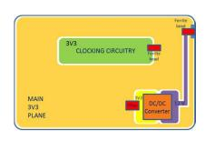
showed a high TIE and period jitter reading on the 99 MHz clock with the shape of the histogram suggesting a high amount of deterministic jitter. The jitter spectrum gives clues about the main source of the jitter. There is a high peak around the 780 KHz and a smaller peak at double this frequency. This corresponds to the switching frequency of the DC/DC converter, LTM4600EV. Therefore, the main jitter contribution comes from the ripple on the 3.3 V output from the DC/DC converter.
