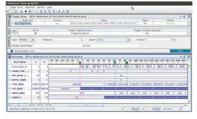
CLOCK AND DATA AFTER 30M CAT6 SFTP CABLE AT THE RECEIVING FPGA INPUT
