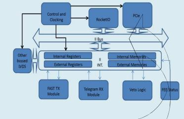
The firmware block diagram for the CC board The FAST TX module generates the FAST data to the FEMs. The telegram RX module receives and decodes the information coming from TR board on a clock and data pair through the
