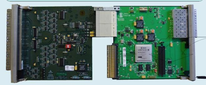
The connections to the FEM boards are realised on AC-coupled LVDS links on CAT5 RJ45 cables. The RTM board provides the number of channels to support up to 16 FEM modules for a 1 MPixel 2D detector.
