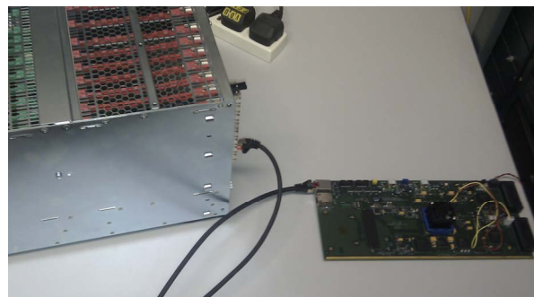
Fig. 11. Experiment setup involving the prototype LPD FEM board
