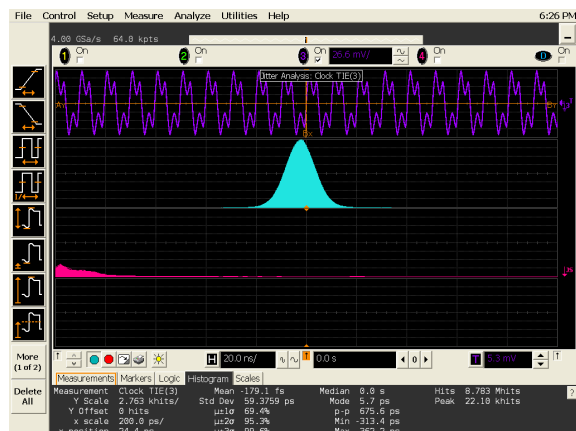
Fig. 7. The TIE snapshot corresponding to the case where 3.3V power is supplied externally.
