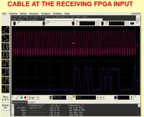
The tests were performed using Ethernet cables of lengths 10m, 15m, 20m, 30m and 50m. There were no errors observed during a period of more than 24 hours with the CAT6 SFTP cables up to 30m. If there is a need to support a 50m cable length MLVDS drivers are going to be tested for data and clock transmission.
