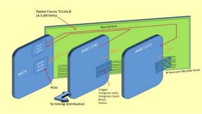
The link between a FEE unit and the CC system consists of 3 LVDS pairs to transfer the 99 MHz clock, FAST data and the VETO information and 1 pair to receive the status information from the unit. One CC RTM can support up to 16 FEE units which in turn support a 1 mega pixel detector. The system is scalable such that by the use of CC slaves in a single 12 slot MTCA.4 crate, up to 6 megapixel detectors can be supported.
