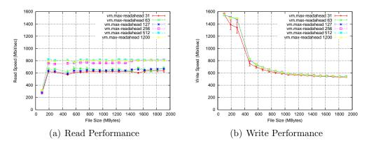
Figure A.2: Performance for ICP SATA (RAID 5 with 4 Disks and 66Mhz PCI).
