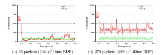
Figure 8.30: H-TCP under asymmetric network conditions (100Mbit/sec capacity, with Flow 1 experiencing 162ms RTT and Flow 2 experiencing 22ms RTT. Bottleneck queue size at 20% BDP of the 162ms flow).
