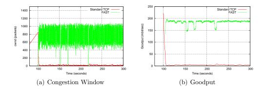
Figure 8.35: Standard TCP competing against FAST under asymmetric network conditions (250Mbit/sec capacity, 42ms RTT, 20% BDP queuesize).
