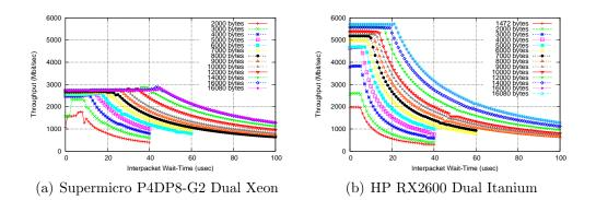
Figure A.11: Throughput performance of 10Gb/sec Intel NIC cards (PCI-X at 133Mhz).
