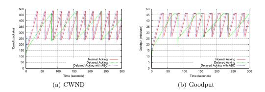
Figure 5.6: Effect of delayed acks upon cwnd dynamics.
