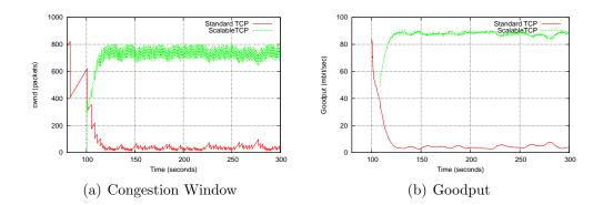
Figure 8.33: Standard TCP competing against ScalableTCP under symmetric network conditions (100Mbit/sec capacity, 82ms RTT, 20% BDP queuesize).
