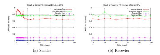
Figure 5.5: Effect of varying TX Interrupt values on CPU load.
