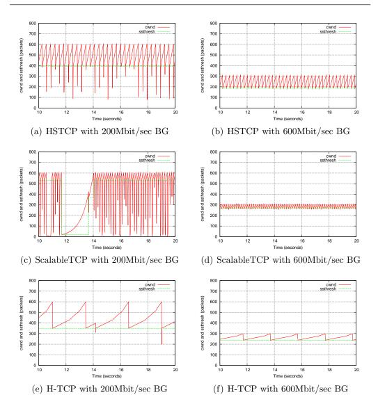
Figure 9.12: *cwnd* trace of New-TCP algorithms with various CBR Background Traffic loads on MB-NG.
