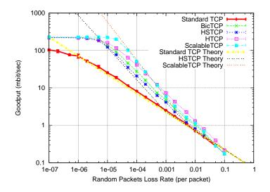
Figure 8.1: Effect of varying the dummynet random loss probability on a single TCP flow (250Mbit/sec, 162ms RTT, Bottleneck queue-size 20% BDP).
