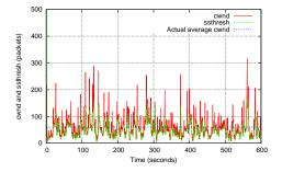
Figure 8.3: H-TCP *cwnd* dynamics showing the mode switch from low-speed into high-speed modes (250Mbit/sec, 162ms RTT, queue-size 20% BDP).
