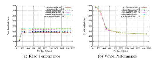
Figure A.1: Performance of ICP SATA (RAID 5 with 4 Disks and 33Mhz PCI).
