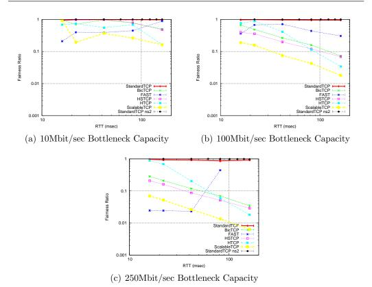
Figure 8.32: Friendliness between a Standard TCP flow competing against a New-TCP flow with symmetric network conditions (Bottleneck Queuesize set to 20% BDP).
