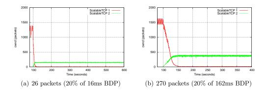
Figure 8.29: ScalableTCP under asymmetric network conditions (100Mbit/sec capacity, with Flow 1 experiencing 162ms RTT and Flow 2 experiencing 16ms RTT).
