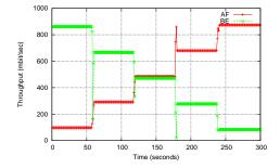
Figure 9.19: Dynamic switching of BE:AF bandwidth allocations every 60 seconds from 90:10, 70:30, 50:50, 30:70 and 10:90.
