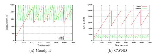
Figure 5.2: Effect of TCP performance with different MTU sizes.
