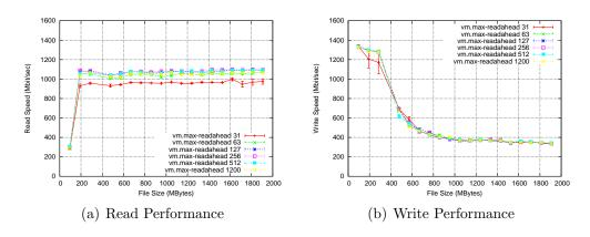
Figure A.4: Performance for 3Ware ATA (RAID 5 with 4 Disks and 66Mhz PCI).
