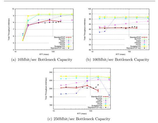
Figure 8.10: Aggregate Goodput of two competing New-TCP flows under symmetric network conditions (Bottleneck Queuesize set to 20% BDP).
