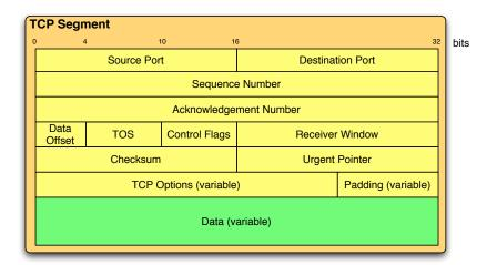
Figure 4.2: TCP header format.
