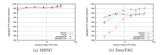
Figure 9.7: Aggregate goodput of n New-TCP flows.
