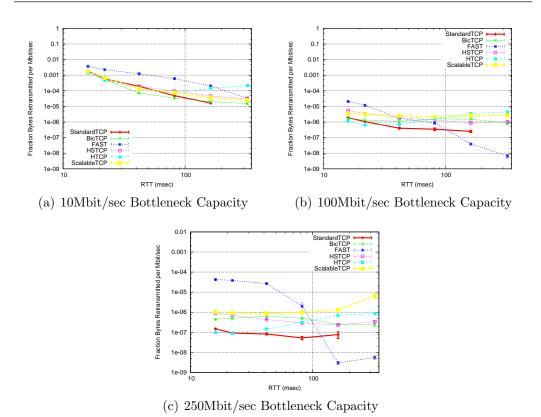
Figure 8.18: Overhead of New-TCP algorithms with two competing TCP flows with symmetric network conditions (Bottleneck Queuesize set to 20% BDP).
