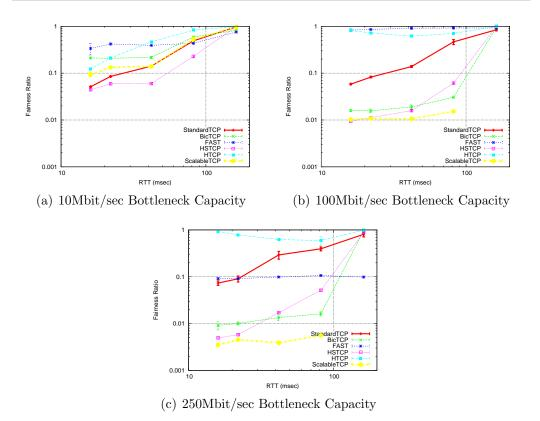
Figure 8.28: Fairness between two competing TCP flows with asymmetric network conditions. The first flow is set to 162ms RTT and the second flow to that as shown (Bottleneck Queuesize set to 20% BDP of the high latency flow).
