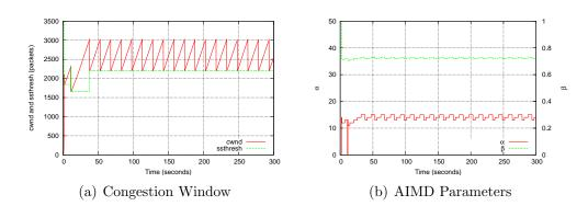
Figure 6.1: *cwnd* dynamic of HSTCP (Single flow on Dummynet, link capacity 200Mbit/sec, RTT 150ms, queue size 500 packets.)
