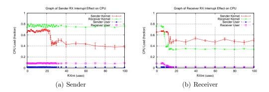
Figure 5.4: Effect of varying RX Interrupt values on CPU load.
