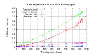
Figure 5.3: CPU utilisation with different TCP throughputs.
