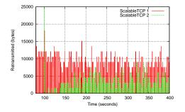
Figure 8.9: Instantaneous retransmissions of ScalableTCP every 100ms at 80% queue size provision under symmetric network conditions. (100Mbit/sec, 82ms RTT).
