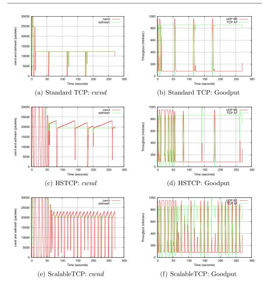
Figure 9.21: New-TCP cwnd and throughput dynamic with 90% AF allocation.
