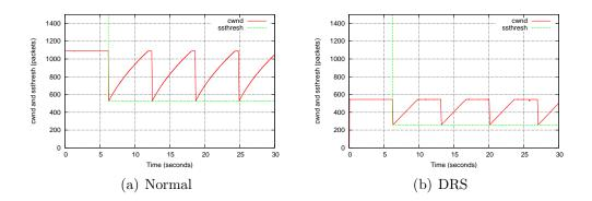
Figure 5.7: Effect on cwnd with Dynamic Right Sizing.
