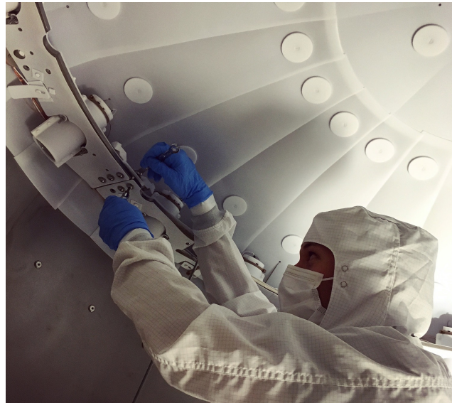
Installation of top skin PMTs
