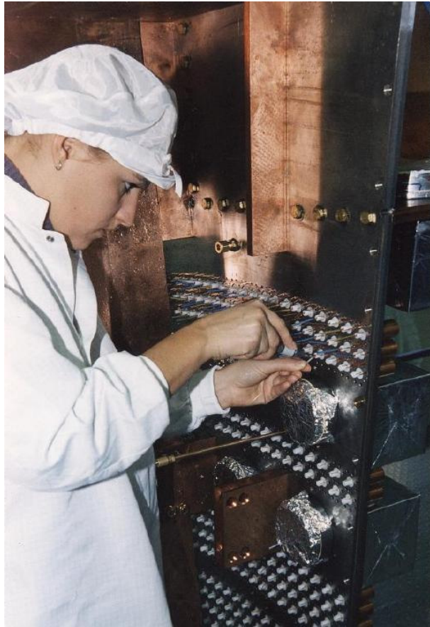
Figure 2.32: Photography of a petal sector during wiring. The operator blocked up the tapered half-cylinder in copper for an anode wire.
