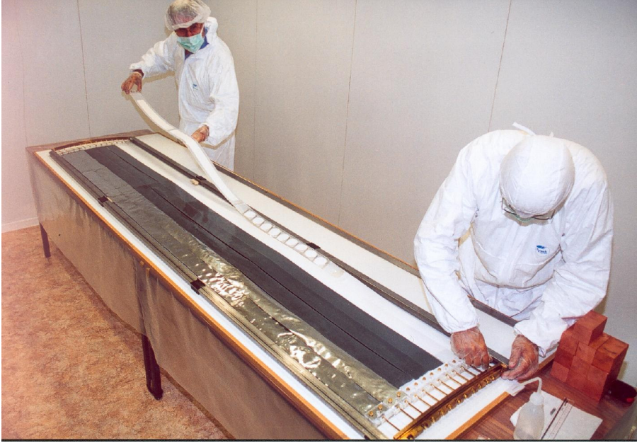
Figure 2.12 : View of source foil production for sector 05, by attachment of the seven strips in the LSM clean room (see the calcium portion' strip with the nine 40 mm diameter disks).
