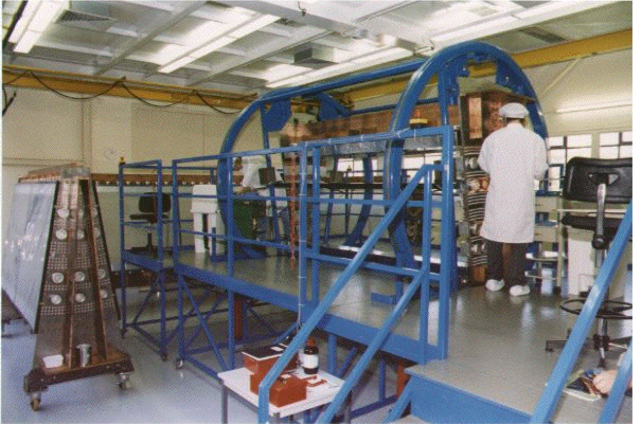
Figure 2.31: Photography of the gimble used for the wiring, installed in the clean room. The gimble was composed of two half-arches for an easy introduction of the sector. It used an electrical system for the 360^\circ rotation and was surrounded by many removable platforms. One can see a sector in the gimble during wiring and on the left side another sector with its protection shields, waiting for bad wire replacement after the test procedure.
