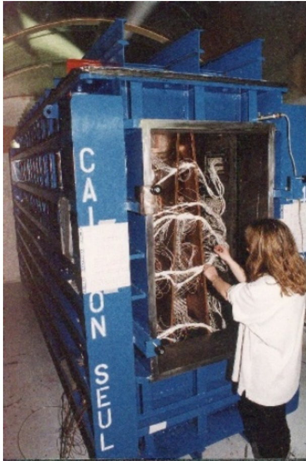
Figure 2.35 : Temporary cabling of one sector in the special container before tests of the wire chamber.
