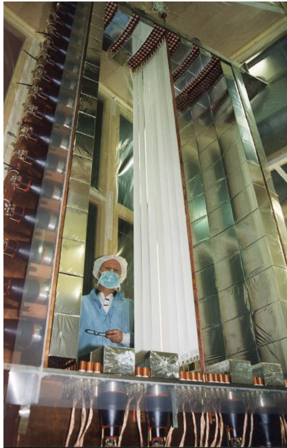
Figure 1.14: View of the third sector in the source mounting room just after the installation of the tellurium source.
