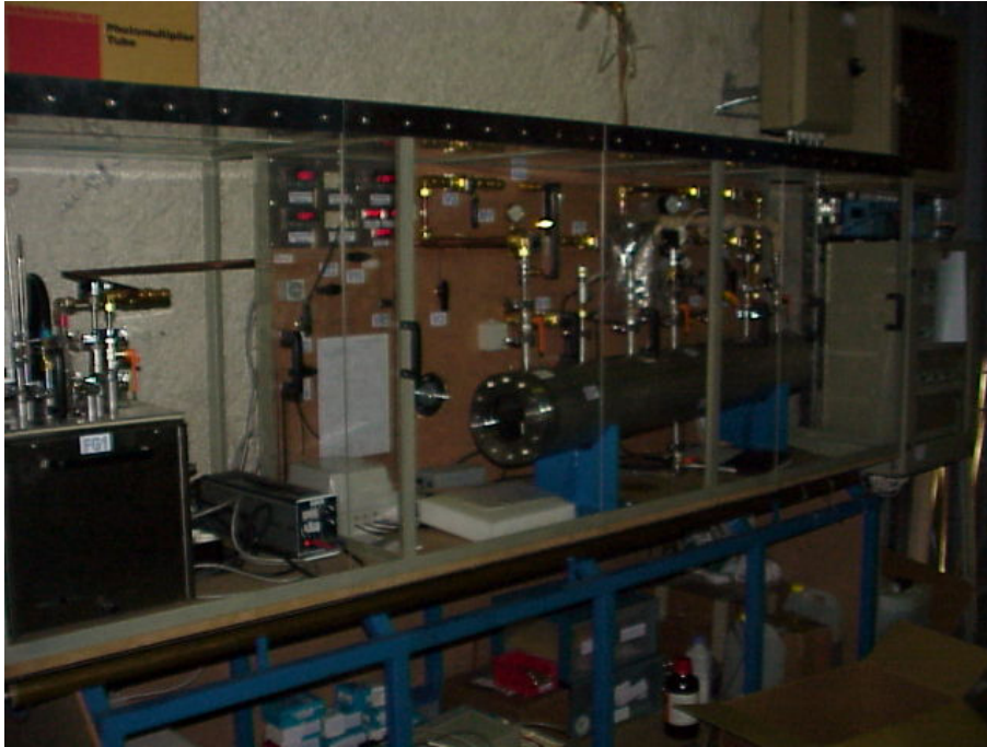
Figure 2.68 : Picture of the gas regulation system for NEMO 3.
