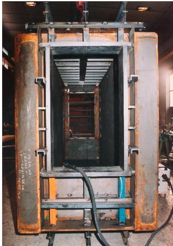
Figure 2.34: Realization of the special container used to test each sector after wiring.
