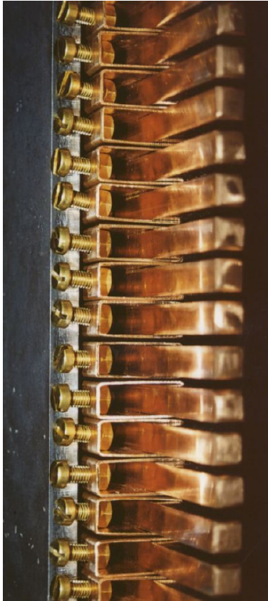
Figure 2.64: Detail of the copper rings used to realize the magnetic coil.
