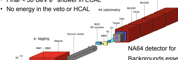
NA64 detector for  $A' \rightarrow invisible$  channel.
